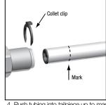
Push tubing into tailpiece up to mark
