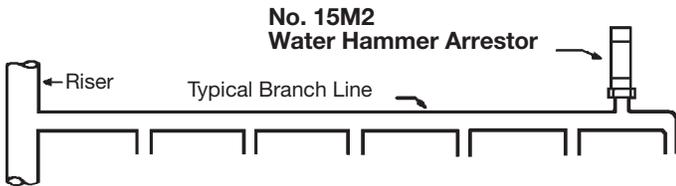
As shown, it has been established that the preferred location for the water hammer arrestor is at the end of the branch line between the last two fixtures served.
