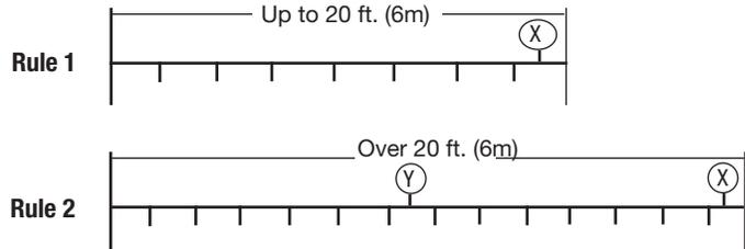
**Rule 1** covers multiple fixture branch lines which do not exceed 20 ft. (6m) in length.
