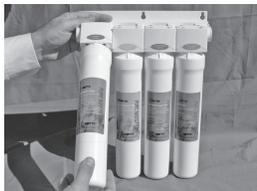
**Step B** – To make the removal of the filter housings easier, the heads & housings may be lifted up to 90 degrees as shown in the pictures to the right. Starting with the sediment filter, lift the cartridge up to 90 degrees. Rotate the cartridge a ¼ turn counterclockwise, remove and dispose of used cartridge.
