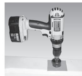
**Step C** – Using a ½" hole saw, proceed to drill the large hole. Keep drill speed on the slowest speed and use lubricating oil or liquid soap to keep the hole saw cool during cutting.
