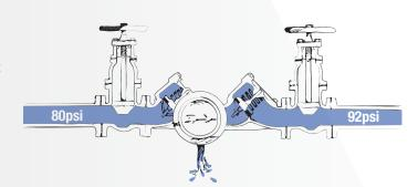
In this figure of an RP device, there is a backpressure condition. The second check is fouled with a piece of pipe scale which permits the higher pressure to flow back into the zone. Here the relief valve discharges the water to atmosphere maintaining the pressure in the zone lower than the supply pressure.
