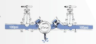
In this view of a pressure vacuum breaker, a backsiphonage condition has caused the check to close against its seat and the air-inlet has opened so that the pressure in the body of the device is atmospheric. If the check was fouled by some foreign material, only air would be pulled back into the domestic supply system instead of the non-potable water downstream of the device.
