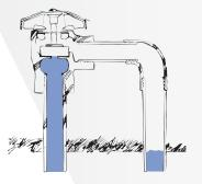
In this view of a double check valve, there is backpressure from a source downstream which has caused the second check to close tightly against this reverse pressure. The first check has closed tightly by itself, thus giving two barriers against the backflow condition.
